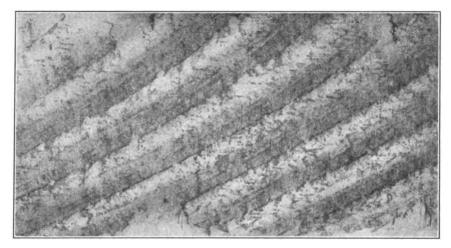
FIG. 3.—RIFLINGS SHOWING TRIPLE THREADS AND LACK OF PARALLELISM DUE TO CHANGING PITCH. (RUB OF CORE.)
